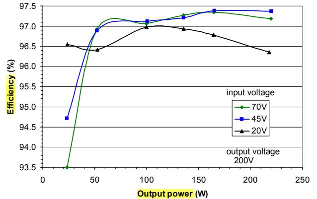
Fig. 13 Experimental results of efficiency as a function of the input voltage and the output power
