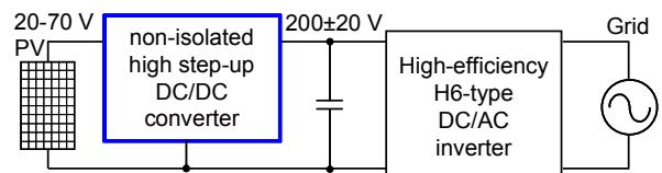
Fig. 1 PV ac module application of the proposed converter
