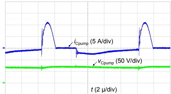
Fig. 9 Experimental waveforms of the pump capacitor current and voltage
