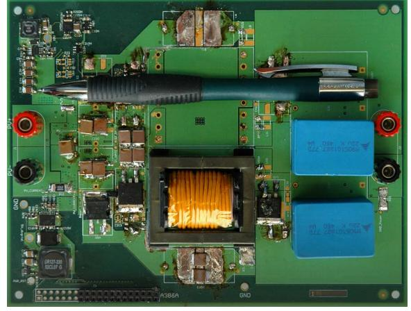
Fig. 7 Prototype photograph of the proposed high step-up converter
