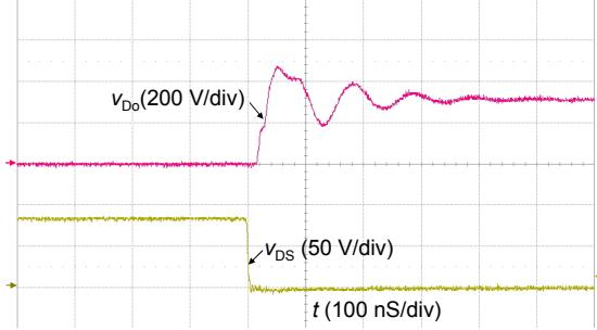
Fig. 11 Experimental results of the output diode voltage stress
