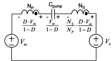
Fig. 5 Simplified voltage loop when output diode is on
