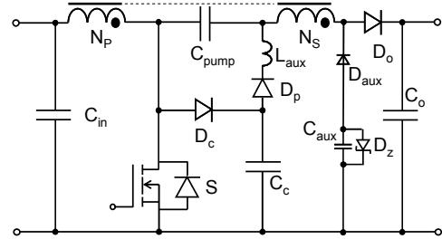
Fig. 8 Implemented circuit of the prototype
