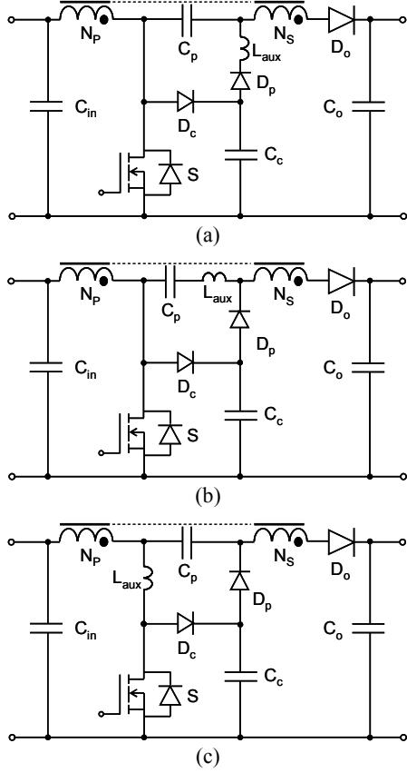
Fig. 6 Three optional places for the insertion of the inductor  $L_{aux}$
