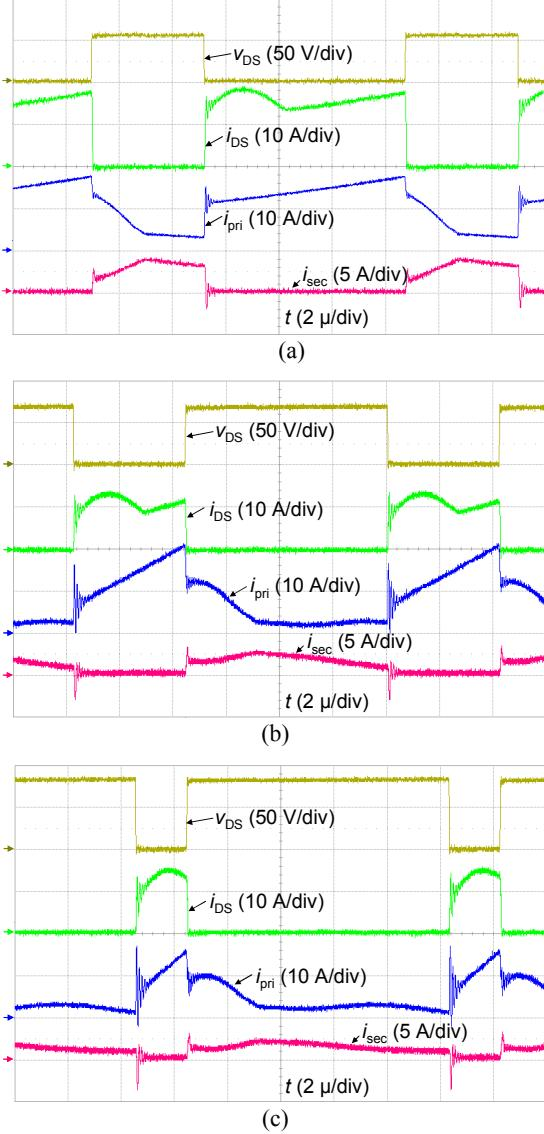
Fig. 10 Experiment verification for active device voltage and current, primary and secondary current: (a) 20V input voltage; (b) 45 V input voltage and (b) 70 V input voltage
