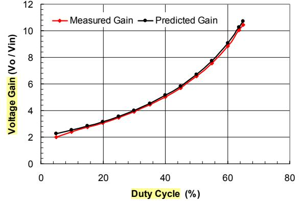
Fig. 12 Measured and predicted voltage gain.
