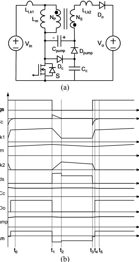
Fig. 3 Basic principle of the proposed converter: (a) equivalent circuit; and (b) key waveforms.
