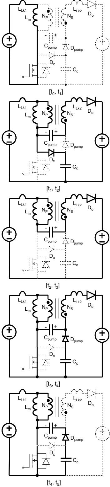
Fig. 4 Topological modes of the proposed converter
