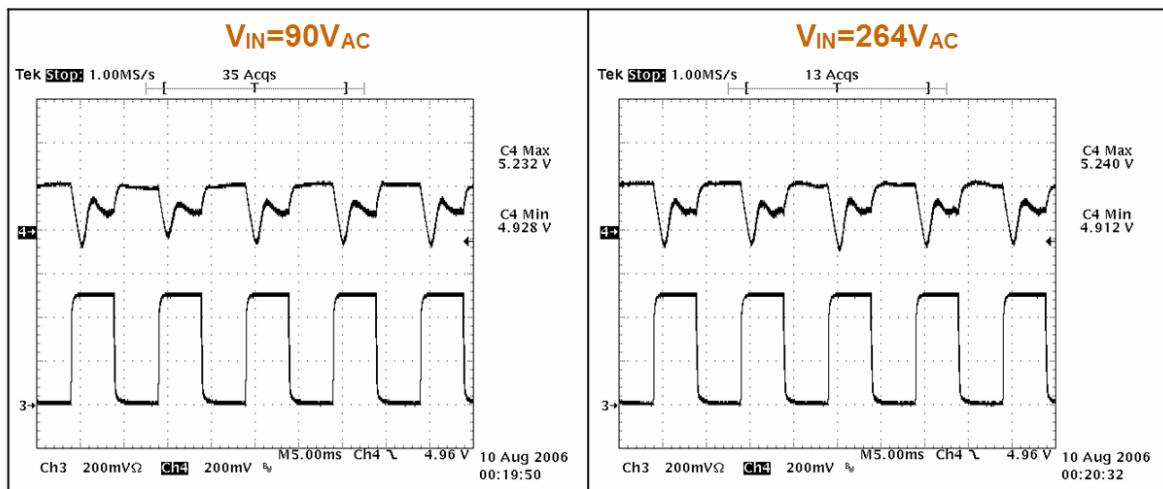
Note: Step Load 0A-0.5A-0A; Slew rate: 0.1A/us
