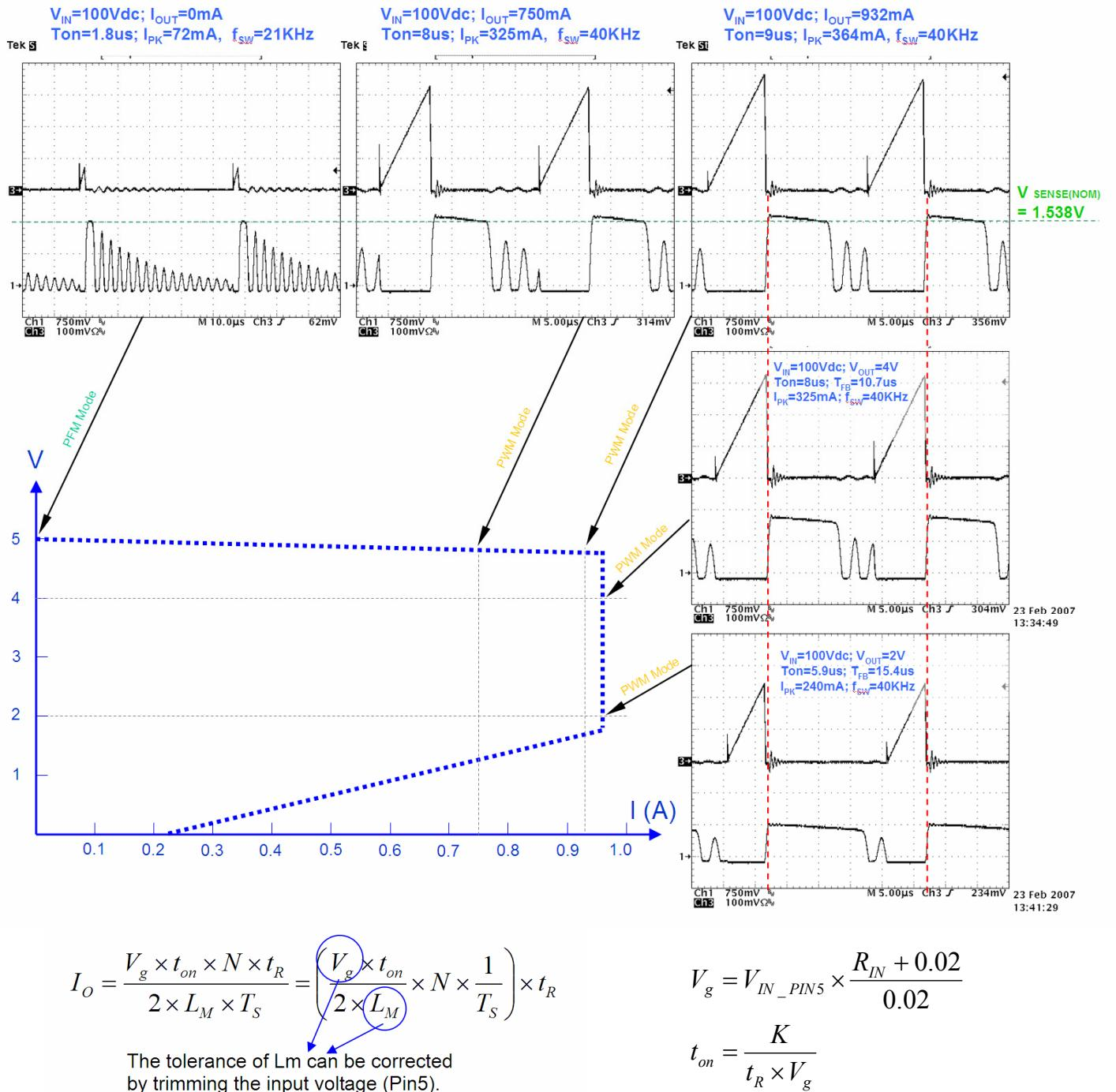
Figure-4, Constant Current Operation
