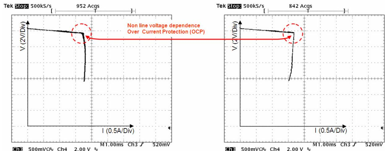
Note: Output voltage is measured at DC cable end.
