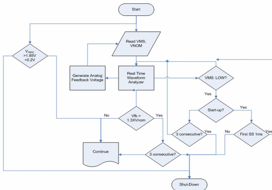
Figure-5, Overvoltage Shutdown Waveforms & Decision Tree
