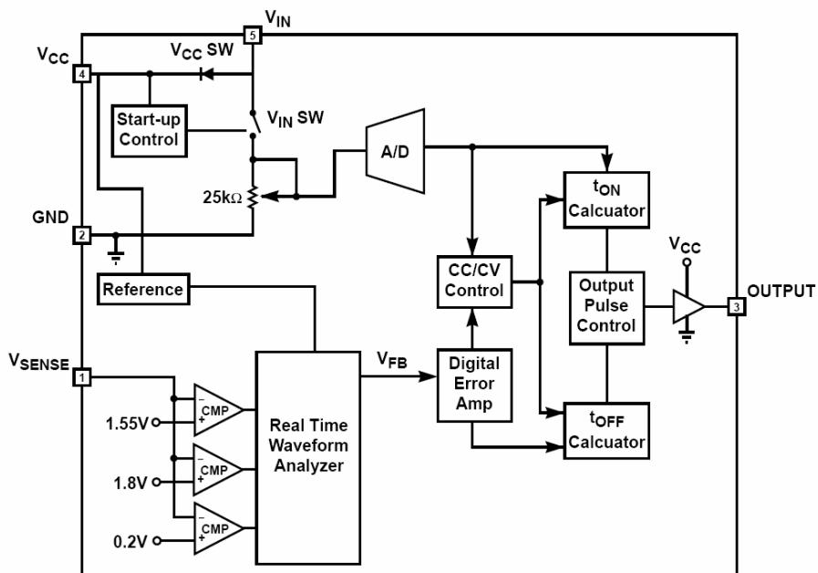
Figure-2, Digital PWM Controller Functional Block Diagram
