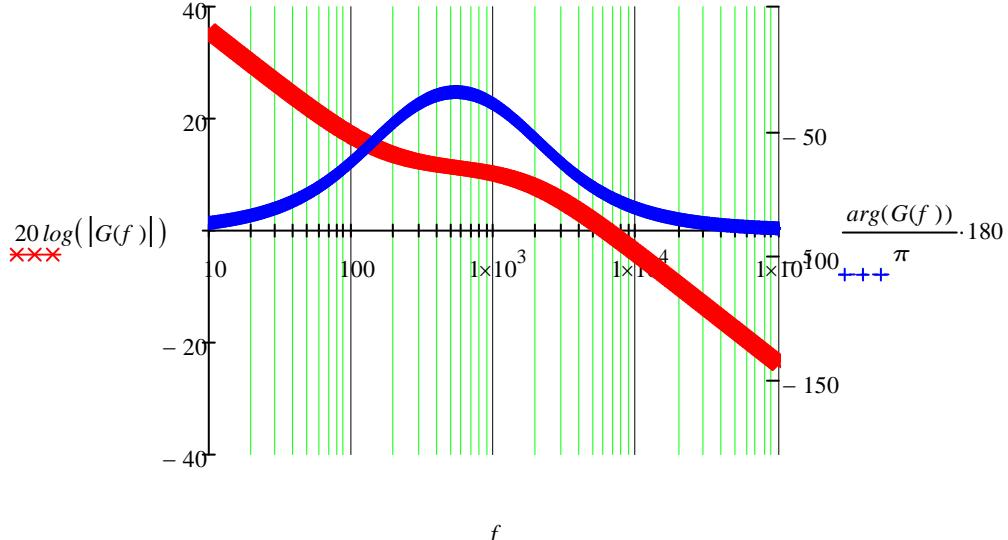
Combining the power stage and compensation circuit in serial:
