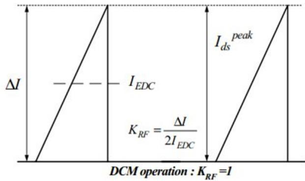
$$I_{EDC} := \frac{P_{in}}{V_{inmin\_DC} D_{max}} = 0.184A$$
